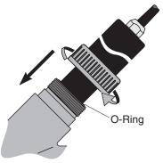
Insert the adapter with the sensor into the flow-thru adapter and tighten the swivel nut. Make sure that the O-ring is inserted in the groove.
